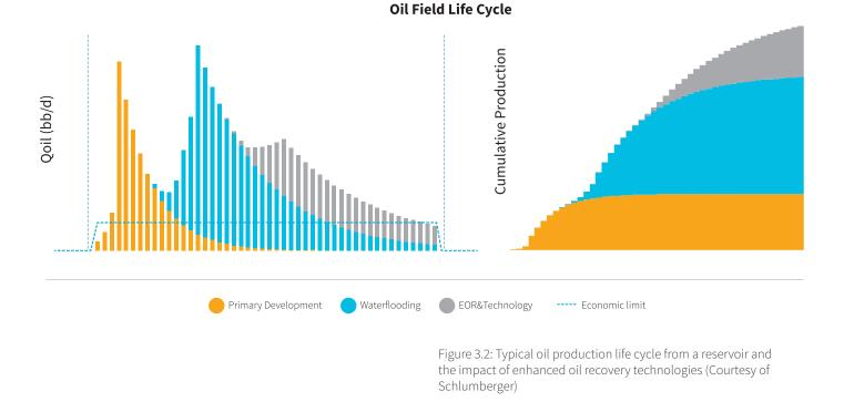
Improved Oil Recovery (IOR) and Enhanced Oil Recovery (EOR) may actually be used at any point in the life of a field, even from the beginning of its development. The IOR and EOR technologies are highly complementary. Ultimately, it is all about optimizing recovery and about energizing the oil in the reservoir to drive more of it to the surface.
