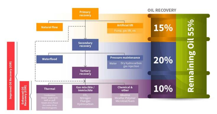
Figure 3.1: Schematic illustration of the IOR/EOR concurrent definition/approach with primary, secondary and tertiary recovery and associated technologies (Modified from 6)
