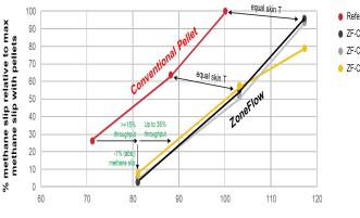
% NG flow rate relative to max NG flow rate tested with pellets
